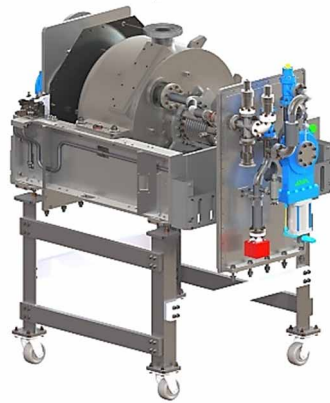
Figure 12: SRF-PI cryomodule coldmass. The alignment rails support the superconducting resonator and solenoid.
