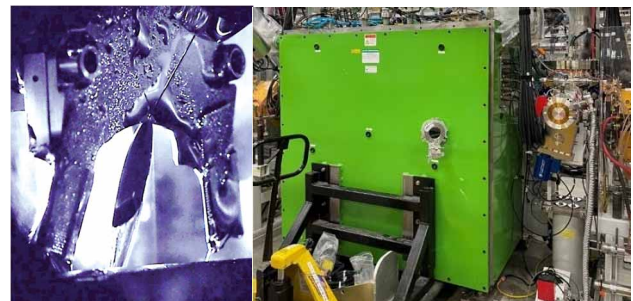
Figure 4: Charge stripper systems: liquid lithium film (left) inside the secondary containment vessel (right, green box) in the FRIB beam line upstream of the rotating carbon foil system (right, on the post).
