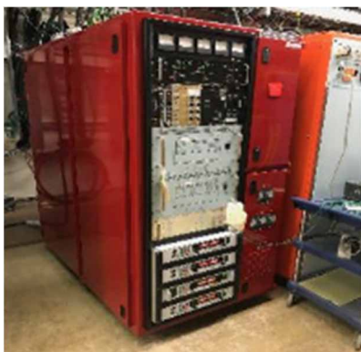
Figure 2: Main Injector Dual-Tube Modulator.
