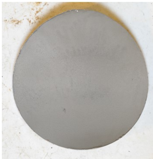
Figure 9: PIE sample cut from test target 1 after January to March 2022 run shows no damage.
