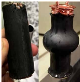
Figure 3: Heat shrink tubing applied on cylinder Cu sample (on the left) and on the 047 cavity (on the right).
