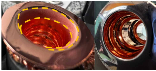
Figure 8: Top cut-off of the 6 GHz cavity after 10 min of PEP treatment. The yellow circles highlight the etched part.
