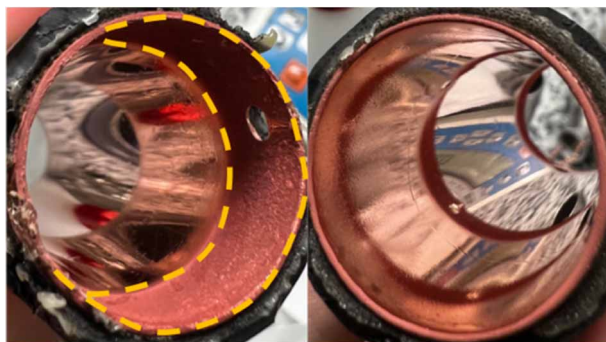
Figure 7: Surface of the cylindrical sample treated with PEP after 7 minutes of processing.
