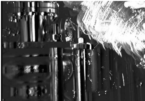
Figure 1: Scattered light of particulates passing through fanned out laser beam during clean blowing. Composite picture of a 15 second video.
