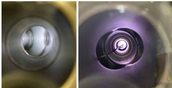
Figure 6: Plasma ignition in 172 MHz HWR cavity. (Plasma ignition is focused in the coupler in the right image from W3 (ref. Fig. 3 for W3 position). A “halo” or “glow” from the plasma in the coupler is seen in the left image, from W1 (ref. Fig. 3 for W1 position)).
