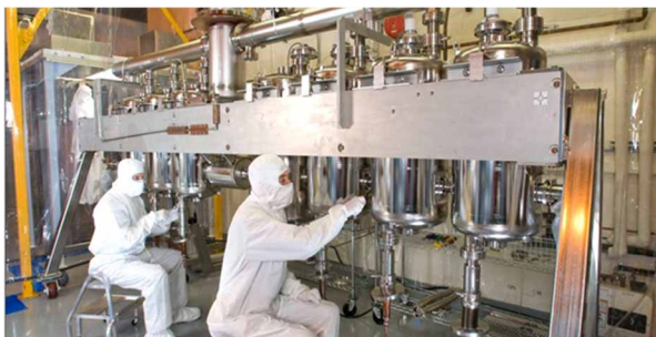
Figure 1: G-Tank upgrade work performed in clean room.
