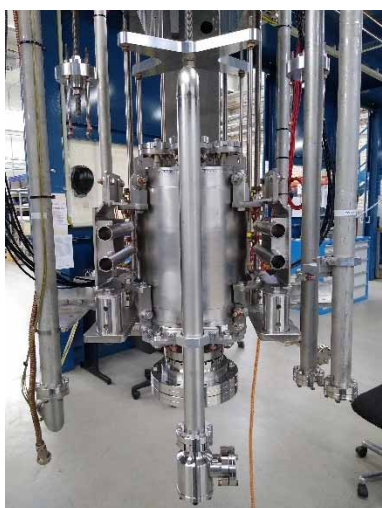
Figure 3: QPR cavity installed to the dedicated insert, which is able to house in addition three single cell cavities.
