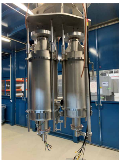
Figure 2: Two 704 MHz cavities installed to one of the dedicated inserts in the AMTF preparation area.
