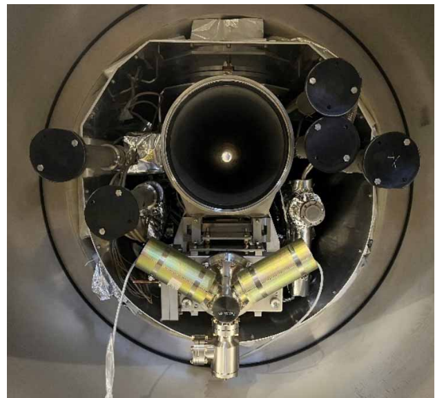
Figure 8: Gauge tree on beamline vacuum.
