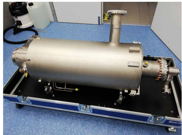
Figure 1: ESS high-beta 704 MHz cavity.
