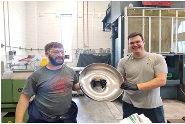
Figure 10: First half cell pressing with aluminum sheet.
