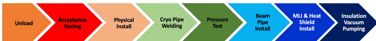
Figure 2: Installation process flow diagram.
