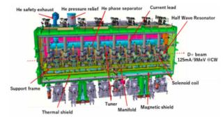
Figure 2: The schematic of the LIPAc SRF cryomodule.
