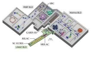
Figure 1: Schematic of the RIBF at RIKEN Nishina Center. The linac facility described in this article is shown in the lower part of the figure.
