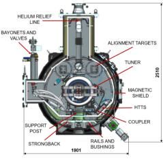
Figure 1: SSR1 CM transverse cross section showing the main components and subsystems (dimensions in mm).
