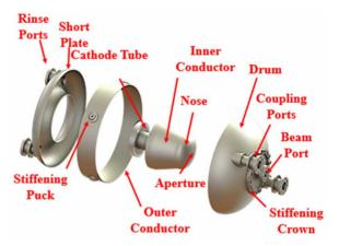
Figure 1: SRF gun cavity with key components.
