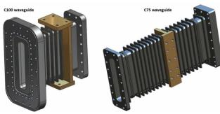
Figure 1: 3D models of C100 and C75 waveguide.
