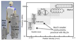
Figure 2: Physical scale of 218 MHz cavity compared to similar geometry 72 MHz cavity in ATLAS. This technology could expand the useful range of different cavity geometries.
