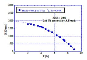
Figure 1: Temperature dependence of  $H_C$  with high purity niobium. The experimental data is from [9]. The T<sup>2</sup> dependence fits the experimental data.  $H_C$  (0) is 1900 Gauss.
