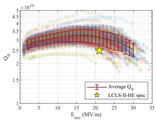
Figure 1: Intrinsic quality factor  $Q_0$  as a function of accelerating gradient  $E_{\rm acc}$  for all production LCLS-II-HE cavities without field emission in vertical test (131 cavities). Red error bars show the average  $Q_0$  with a  $\pm 1\sigma$  interval, up to an arbitrary limit of 30 MV/m.
