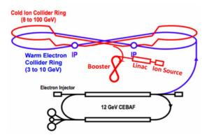
Figure 1: Schematic of Jefferson Lab Electron-Ion Collider.
