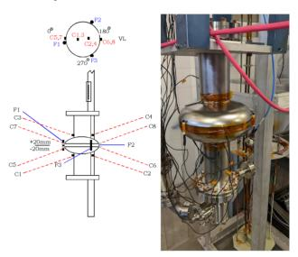
Figure 1: Illustration of the test setup. Left-hand diagram shows the positions of the thermometers (C) and magnetometers (F). Right-hand photo shows the instrumented cavity on the test insert.
