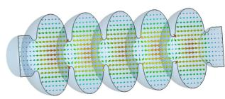
Figure 1: CST model of the 915 MHz five-cell cavity design, the arrows indicated the electrical field in  $\pi$  mode.
