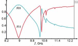
Figure 1: Measured S-parameters of a ZrO<sub>2</sub> sample.
