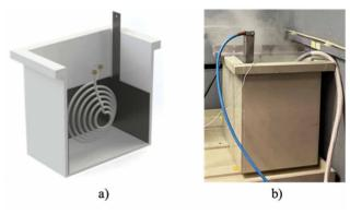
Figure 1: a) A schematic render of the plastic bath used for PEP; b) Photo view during PEP process.
