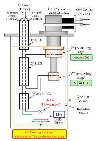
Figure 1: Schematic of RJT-100 4KGM-JT cryocooler.
