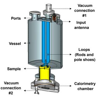
Figure 1: Cross-sectional view of the UHH QPR.
