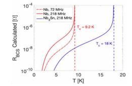
Figure 1: Predicted BCS surface resistance of Nb and Nb3Sn vs operating temperature for two frequencies.
