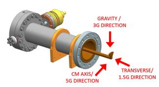
Figure 1: pHB650 coupler vacuum side assembly.
