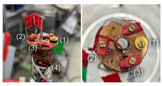
Figure 1: Photographs of the experimental setup. A copper plate is mounted onto the cryo-cooler on which the Cernox sensor (1) and semiconductor components (2)&(3) are screwed. The heater foil (4) is glued onto the cryo-cooler below the plate.
