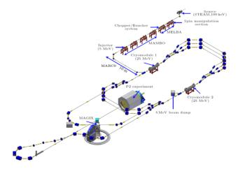
Figure 1: Layout of MESA. A normal-conducting preaccelerator injects a 5 MeV CW beam into the recirculating main accelerator. Two cryomodules accelerate the beam. In external beam mode for the P2 experiment a 150 mA beam is recirculated thrice to a energy of 155 MeV and dumped afterwards.For the ERL experiment MAGIX 1 mA is recirculated twice up to 105 MeV. Afterwards the beam is decelerated in the main accelerator down to 5 MeV.
