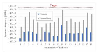
Figure 3: Resonant frequency distribution of niobium halfcells.
