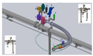
Figure 3: One channel of the purging line with the purging head assembly connected to the main vacuum line.
