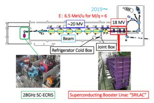
Figure 2: Schematic of the heavy-ion linac facility at RIKEN after the upgrade. The eight tanks shown in yellow are the existing room-temperature drift-tube linac, RILAC.
