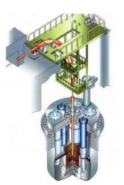
Figure 1: Schematic view of the JAEA-ADS subcritical reactor.
