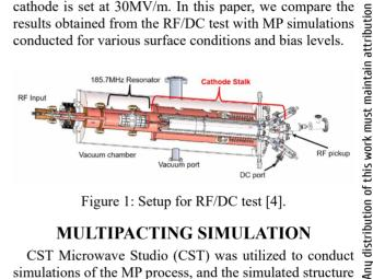
Figure 1: Setup for RF/DC test [4].
