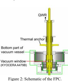
posed of bulk copper and copper-plated stainless steel, respectively. A thermal anchor was connected to a thermal shield cooled using liquid nitrogen.
