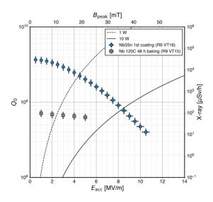
Figure 2: Q - E curves measured at 4.2 K for the single-cell cavity before and after first coating.
