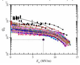
Figure 1: VTA cavity performance with FRIB beta 0.53 half wave resonator (HWRs).
