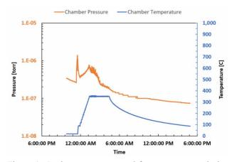
Figure 1: Cavity temperature and furnace pressure during the mid-T baking.
