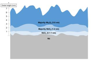
Figure 1: Cartoon of the native niobium oxide structure, taken from [4].
