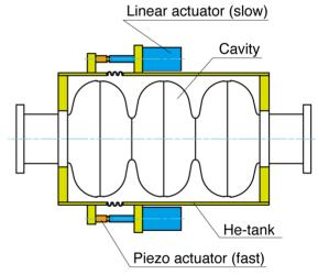
Figure 1: Schematic view of new tuner mechanism.
