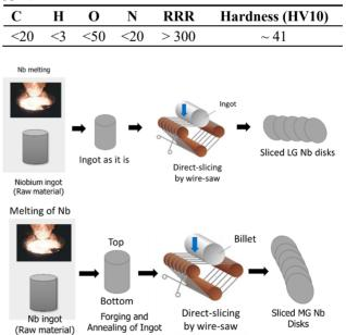
Figure 1: LG Nb manufacturing process (up) and ATI MG Nb manufacturing process (below) [3, 4].
