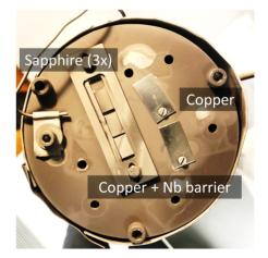
Figure 1: Flat samples right after the coating process, still mounted on the sample holder.
