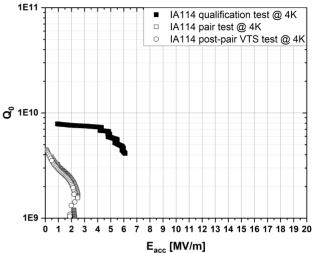
Figure 1:  $Nb_3Sn$ -coated cavity performance before and after the first  $Nb_3Sn$ -coated cavity pair assembly. Note the increase in the low-field surface resistance and strong field dependence in the pair test and the test after the pair assembly.
