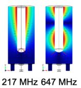
Figure 2: Field distributions for the QWR. Image courtesy of Ref. [6].
