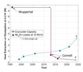
Figure 1: Progress in both  $Nb_3Sn$  cavity performance (red squares) and pulse-tube cryocooler capacity at 4.2 K (blue curve) [10].
