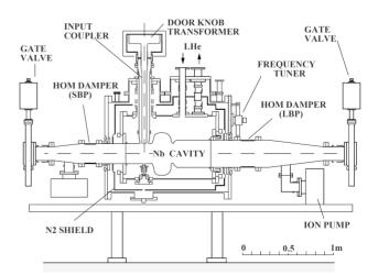
Figure 1: Cross-sectional view of HOM damped SCC designed for KEKB. This cavity is used for SuperKEKB. Ferrite HOM dampers are equipped on both SBP and LBP. The SBP and LBP diameters are 220 mm and 300 mm, respectively.
