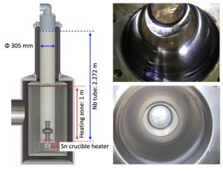
Figure 1: Cross-section of coating furnace (left), inside of cavity before (top right), and after first coating (bottom right).
