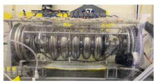
Figure 1: EP tool with a 650 MHz 5-cell cavity.
