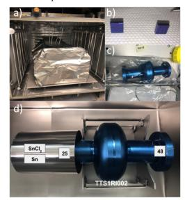
Figure 1: Experimental setup for Nb<sub>3</sub>Sn coating. [a] Assembled experimental setup in the hot zone of the furnace. Note niobium foil covering the assembly and thermocouples at the top. [b,c] Niobium samples (b) and niobium cavity (c) prepared for the coating. Note that the blue color is due to 30 V anodizing. [d] Niobium cavity assembled for the coating inside niobium box on the niobium support fixture.
