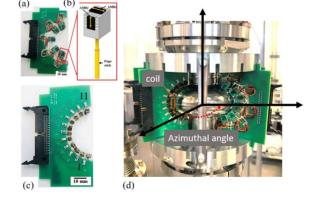
Figure 1: (a) and (b) AMR sensors and (c) temperature sensors board, (d) assembled on the surface of cavity [13].
