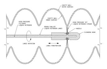
Figure 1: Concept of a high pressure liquid nitrogen jet stream cleaning a cavity surface [3].
