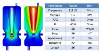
Figure 3: Cavity field distributions and EM parameters.
