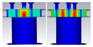
Figure 1: Simulated maps of electric (left) and magnetic (right) RF field for the operational  $TM_{020}$  mode at 4.8 GHz.
