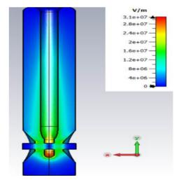
Figure 1: Field map of an FRIB  $\beta = 0.041$  QWR from eigenmode simulation in CST Microwave Studio. Field map represents the operational gradient.
