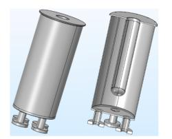
Figure 1: 3-Dimensional computer model of the QWR: Full cavity (left) and cut out (right). This model was generated using COMSOL Multiphysics <sup>®</sup>.
