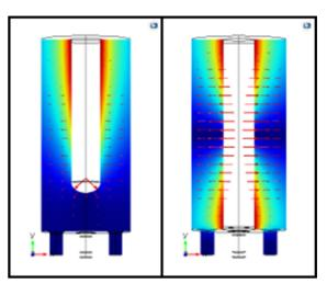
Figure 1: Field Distribution of QWR and HWR.
