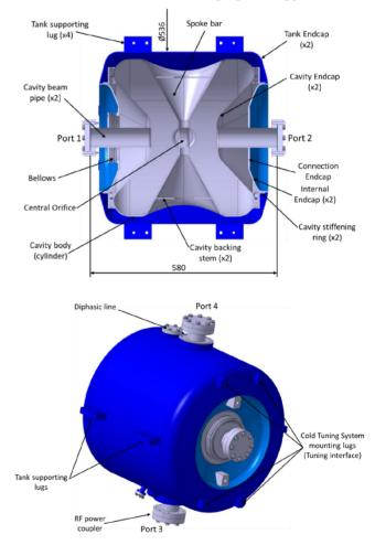
Figure 1: Cross-section and isometric overview of the Single Spoke RF Cavity for MINERVA; the niobium bare cavity is shown in grey, whilst the titanium helium tank is shown in light blue (Courtesy of IJCLab).
