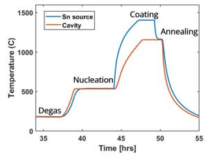
Figure 1: Vapor diffusion temperature profile at Cornell University showing the temperatures of the Sn/SnCl<sub>2</sub> source and Nb substrate (cavity) versus time. The main three stages of coting are nucleation, coating, and annealing.
