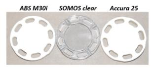
Figure 1: Flanges in ABS M30i, SOMOS watershed with clear coating, Accura 25.
