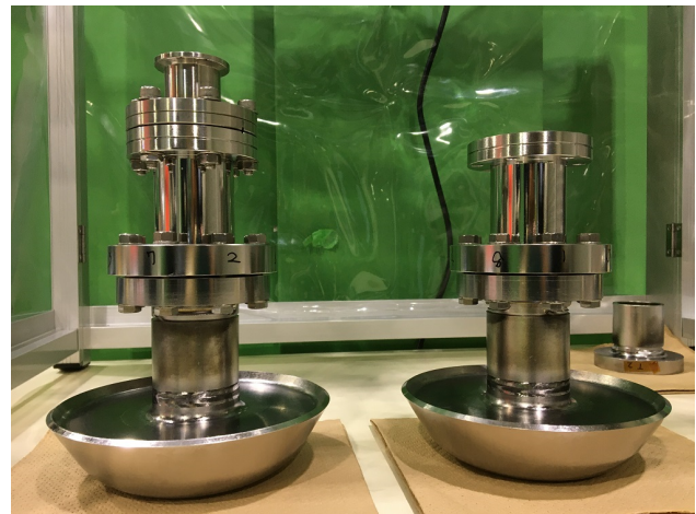
Figure 11: The beam-port assemblies of the prototype spoke cavity fabricated in fy2022. Short pipes for vacuum leak test are attached.
