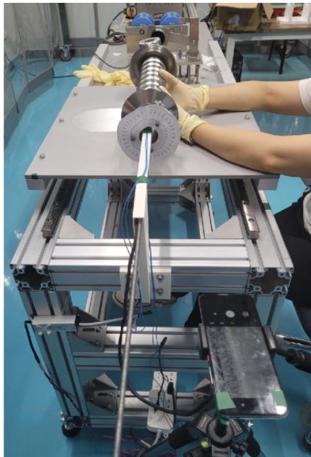
Figure 6: Borescope system of the 3.9 GHz prototype.
