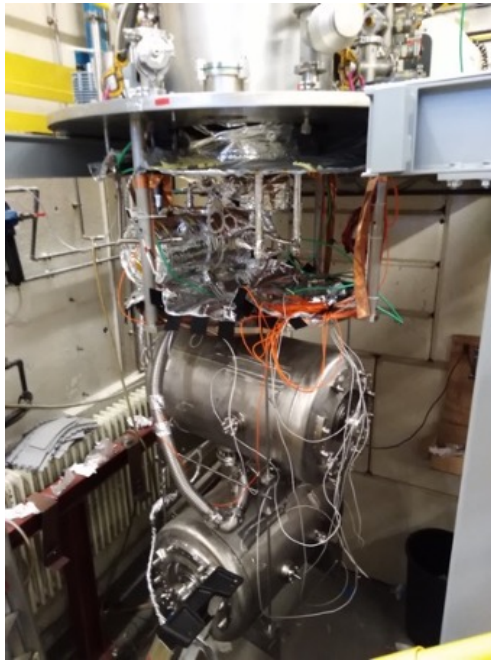
Figure 1: Vacuum insert of the vertical cryostat at SUPRAT-ECH. Two cavities are mounted in the same insert and share the same beam vacuum.
