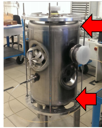
Figure 2: Configuration of the frequency measurement before the trimming and final electron-beam welding. The red arrows indicate the trimming margins and the end-caps are temporarily clamped for the RF measurement at warm.
