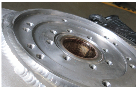
Figure 10: Photograph of the RF port of a \beta = 0.54 HWR after coupler plasma ignition with a copper antenna.
