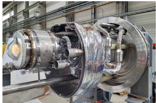
Figure 7: The ACC3 end cap being manufactured at DESY before the 2022 shutdown.
