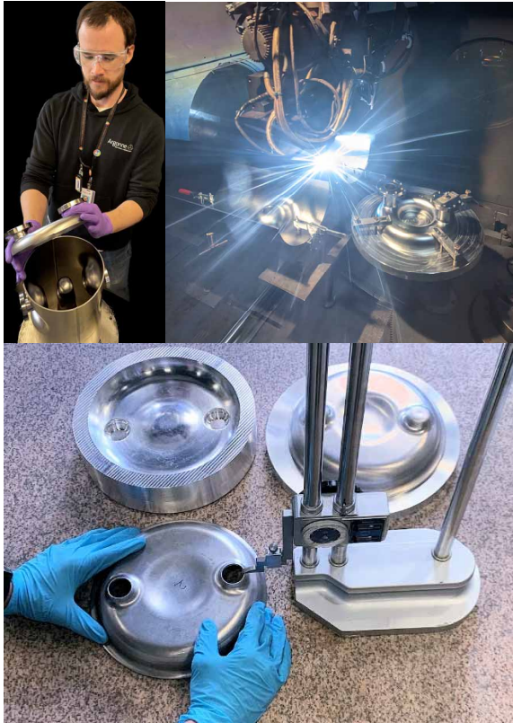
Figure 4: Cavity parts during fabrication (left, bottom) and electron beam welding (right).
