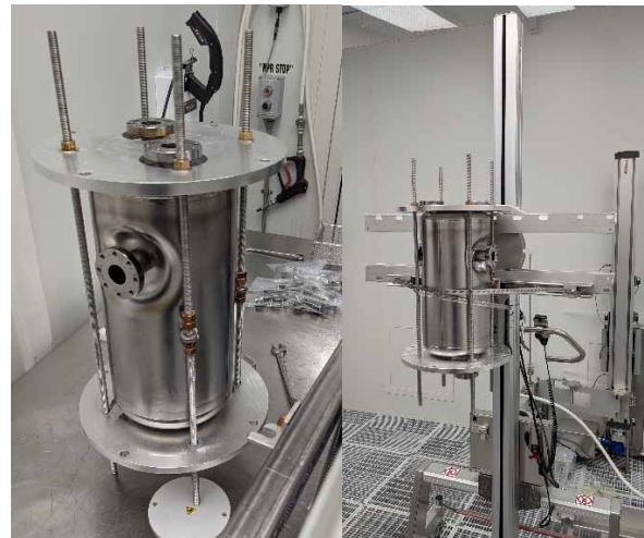
Figure 6: Cavity fixturing used for ultrasonic cleaning and high pressure rinsing.
