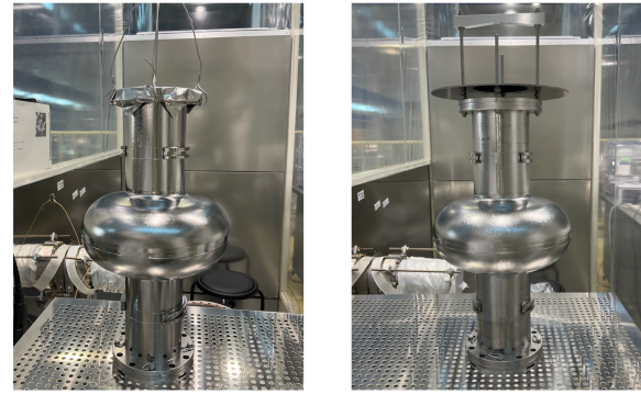
Figure 9: Setup of the cavity for third coating (left) and fourth coating (right).
