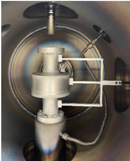
Figure 2: Al-made mock-up cavity and sample holder used for deposition conditions optimization.
