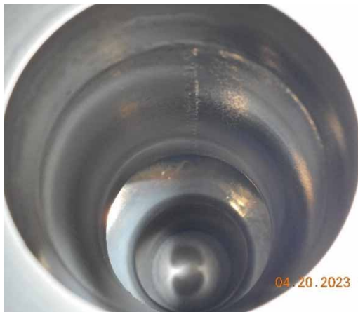
Figure 4: Pictures of post-annealed picture of Nb 3 Sn coated 2.6 GHz Nb cavity (TTS1RI002).
