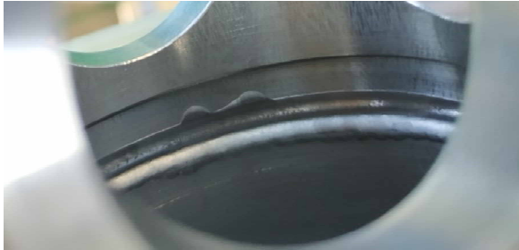
Figure 2: Fully treated weld next to the BPM.
