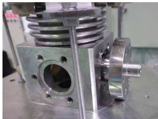
Figure 9: Solenoid V06 faulty BPM pick-up.
