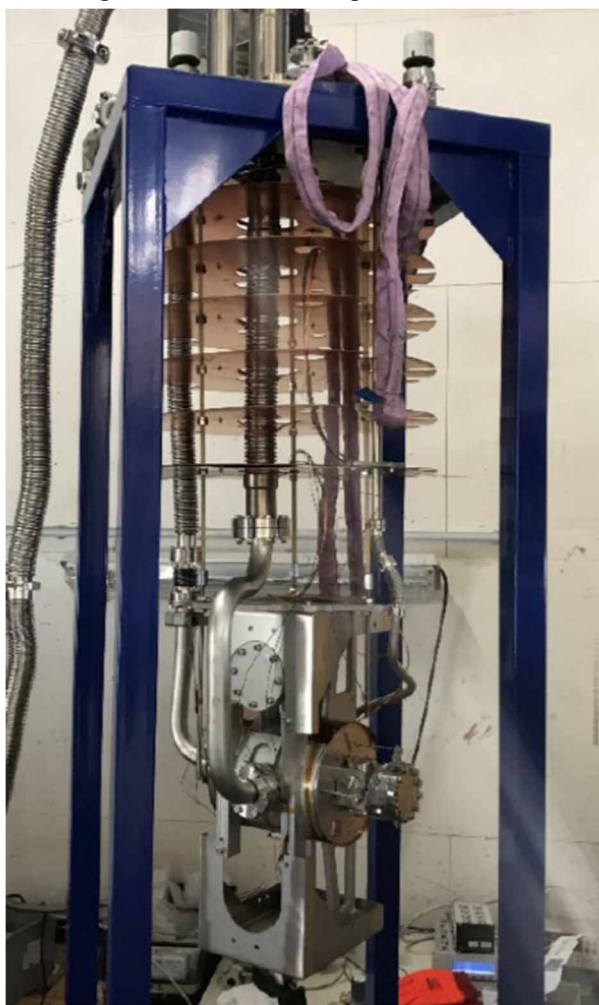
Figure 6: Solenoid installed on the test insert.
