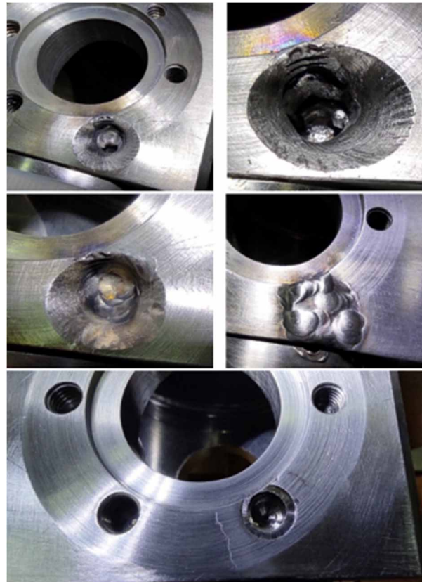
Figure 5: Threaded hole at different stages of charging and its final result (bottom picture).
