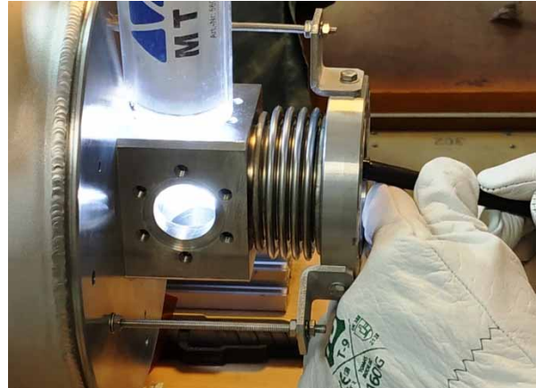
Figure 4: Welding of the new bellow on solenoid V06.
