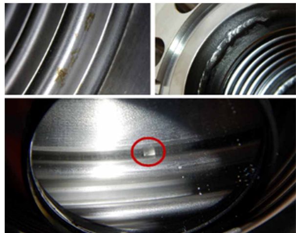
Figure 1: From top right to bottom, rust dots on bellow, oversized weld seam, trapped material in bellow.
