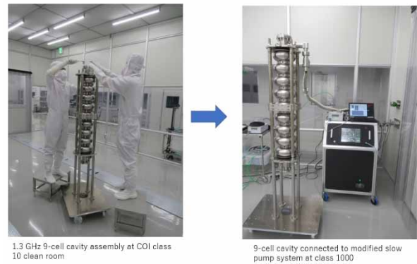
Figure 3: (Left) Assembly work of 9-cell cavity to the modified slow pumping system without HPR. (Right) setup of the slow pumping system with 9-cell cavity.
