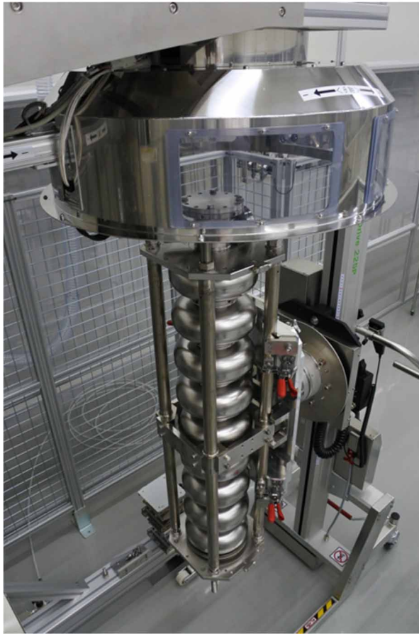
Figure 1: Vertical automatic cleaning system with an installed 9-cell cavity.
