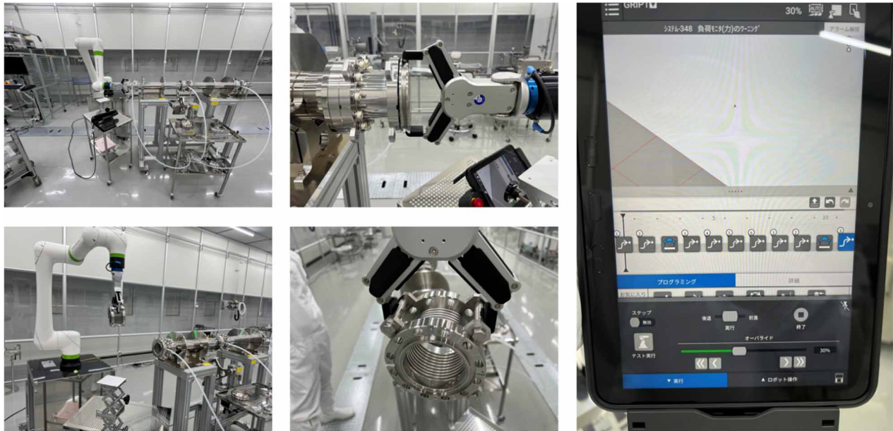
Figure 5: Demonstration of auto-assembly for a blank flange and a connection bellows by a robot arm including program developed on the control panel.
