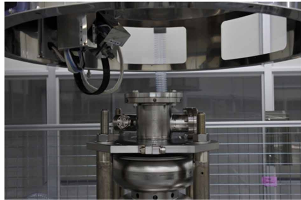
Figure 1: Vertical automatic cleaning system with an installed 9-cell cavity.
