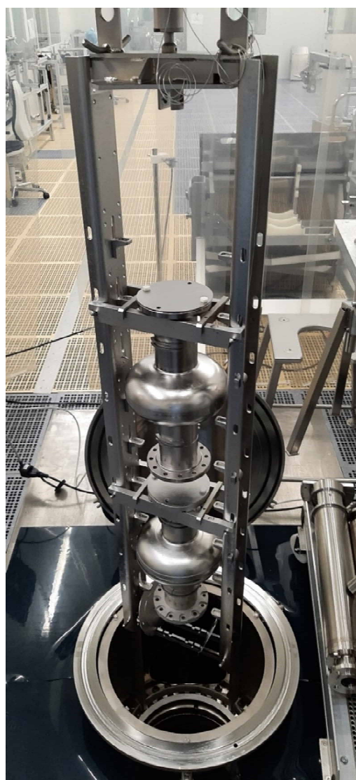
Figure 6: Furnace frame equipped with two since-cell cavities.
