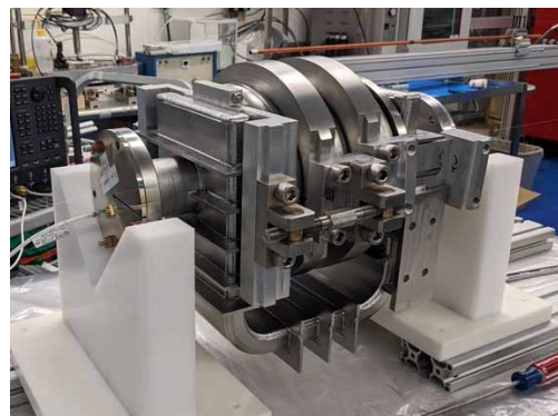
Figure 6: Tuning hardware on the 3-cell.
