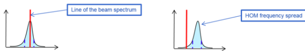
Figure 6: Stochastic HOM excitation by the pulsed beam, resonance (left) and off-resonance (right) case.
