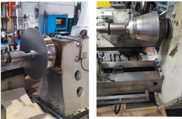
Figure 4: (Left) spinning of drum, (right) spinning of Inner conductor.
