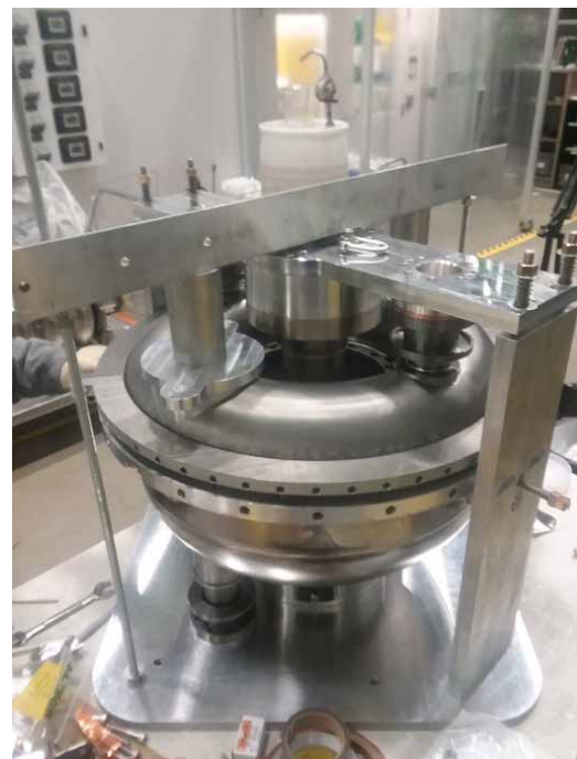
Figure 6: Stack-up/frequency measurement tooling.
