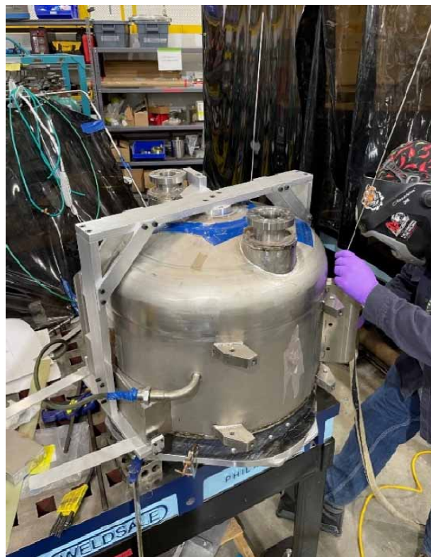
Figure 9: Tungsten Inert Gas (TIG) welding of cavity helium vessel.
