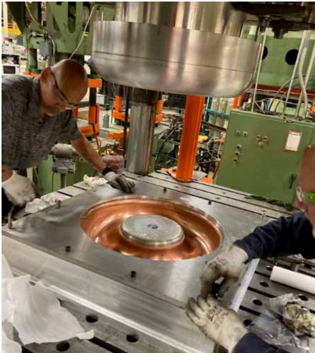
Figure 3: Deep-drawing of short plate ~600 tons.
