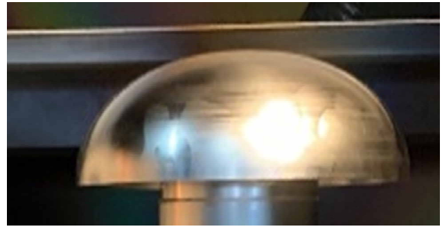
Figure 2: Cavity nose fabricated from large grain ingot slice.
