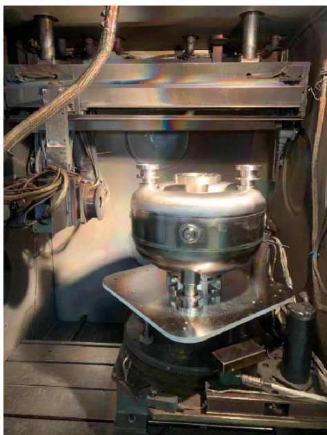
Figure 7: Final conduction mode (full-penetration) weld.
