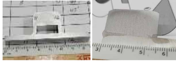
Figure 5: Keyhole weld development for stiffening elements; verifying penetration depth.
