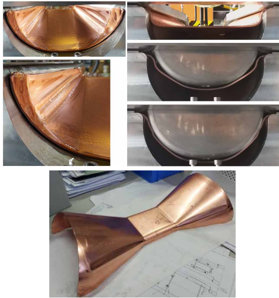
Figure 8: Option A process for half-spokes: copper trials.
