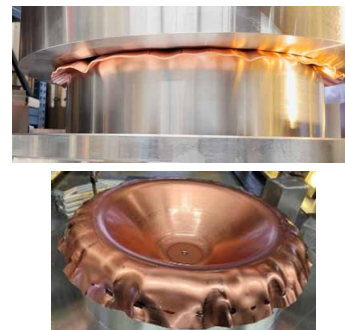
Figure 18: Copper trials of endcap deep-drawing.
