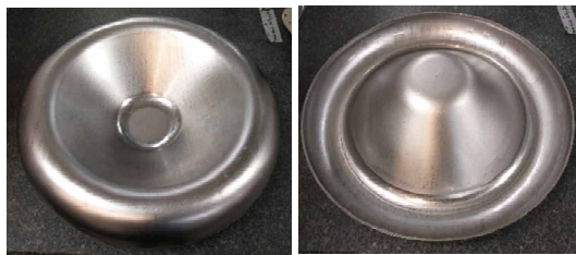
Figure 21: Successful deep-drawing of a niobium endcap.
