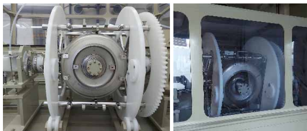
Figure 24: Rotational BCP of the first MINERVA cavity: installation of cavity in the facility (left) and during the process (right).
