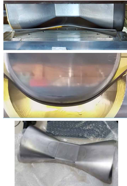
Figure 11: Deep-drawing of niobium half-spoke: view from the side and the extremity during the process and finished part.
