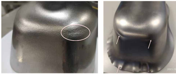
Figure 2: Detail of an RFD Pole showing excessive local thinning, orange peel and wrinkles. Courtesy Zanon and FNAL.
