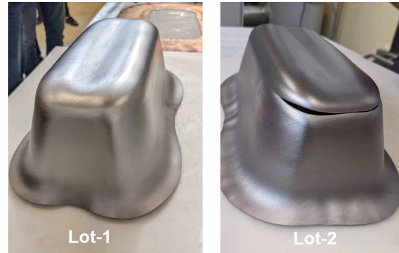
Figure 4: Deep drawing comparison with two material lots. Lot-2 shows a big crack on the upper part of the Pole (corner) as well as wrinkles in the base.
