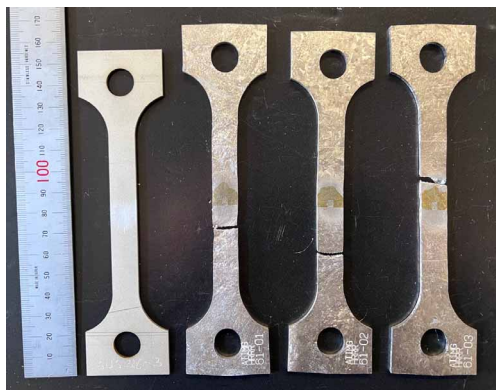
Figure 5: Mechanical properties of various grades Niobium in Liquid helium (up); MG Nb annealed specimens tested in liquid helium (below).
