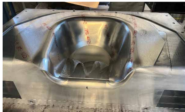
Figure 13: A forming die after stamping an aluminum test part.
