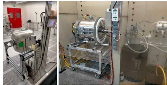
Figure 1: Photographs of a SSR2 cavity installed on HPR unit (left) and on rotational BCP cart (right) on Supratech platform at IJCLab.
