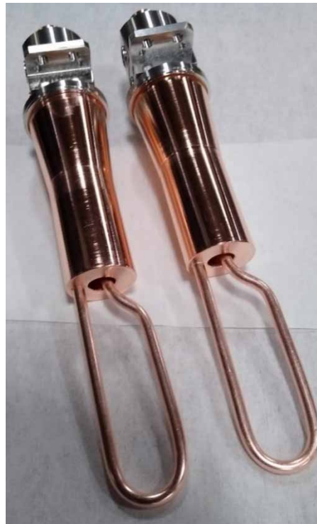
Figure 3: FPC coupling loops installed on the 56 MHz superconducting resonator.
