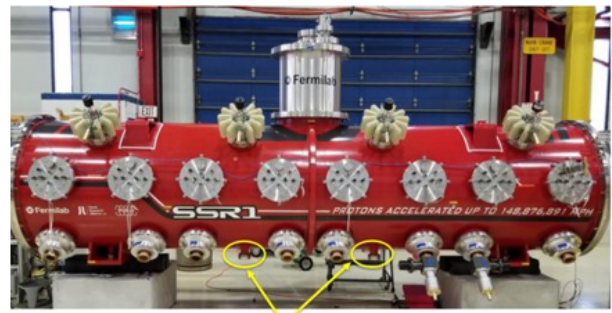
8 heaters: one for each cavity
