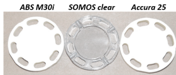
Figure 1: Flanges in ABS M30i, SOMOS watershed with clear coating, Accura 25.
