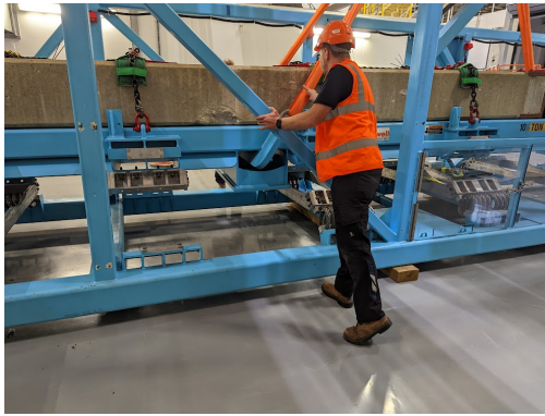
Figure 4: Dummy Load being installed into the Transport Frame at STFC-UKRI.
