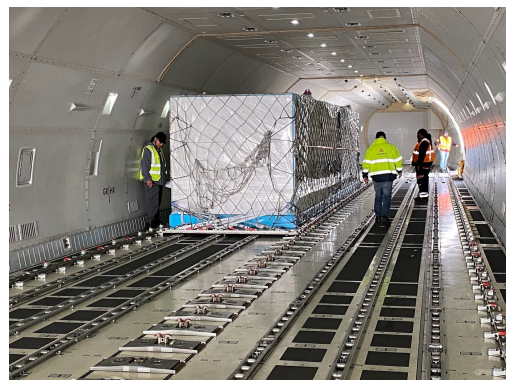
Figure 7: Loading of the frame onto plane, including scissor lifts (top) and universal floor bearing and powered movers (bottom).
