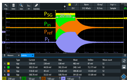
Figure 8: RF signals observed during the pulsed RF power conditioning. P_{SG} , P_{in} , P_{ref} , and P_t are the input pulse from SG, the forward signal from the directional coupler, the reflected signal, and the signal from the cavity pickup, respectively.
