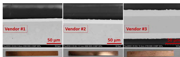
Figure 2: Coupons from three plating vendors: 1) RRR coupons, 2) cross section by SEM.
