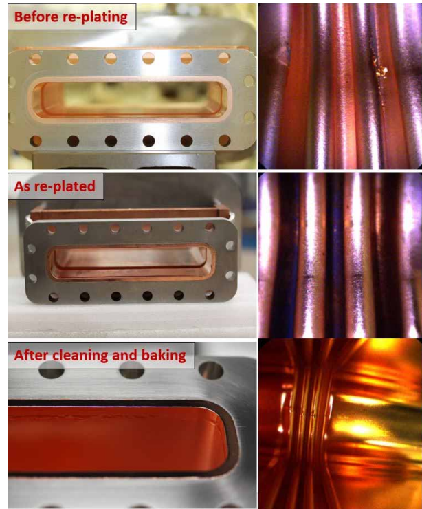
Figure 6: Sample C100 waveguide before re-plating, as re-plated, after cleaning and baking.
