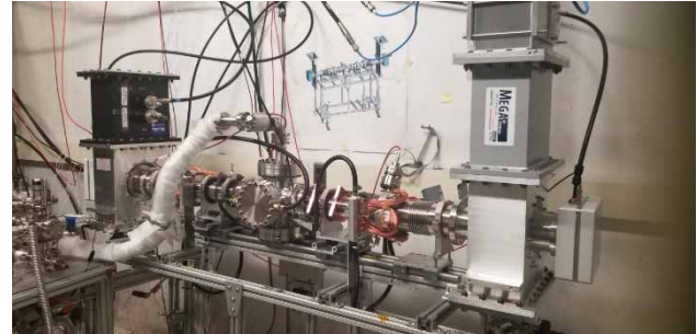
Figure 5: Warm RF test stand for qualification of two 650 MHz couplers in SW regime.
