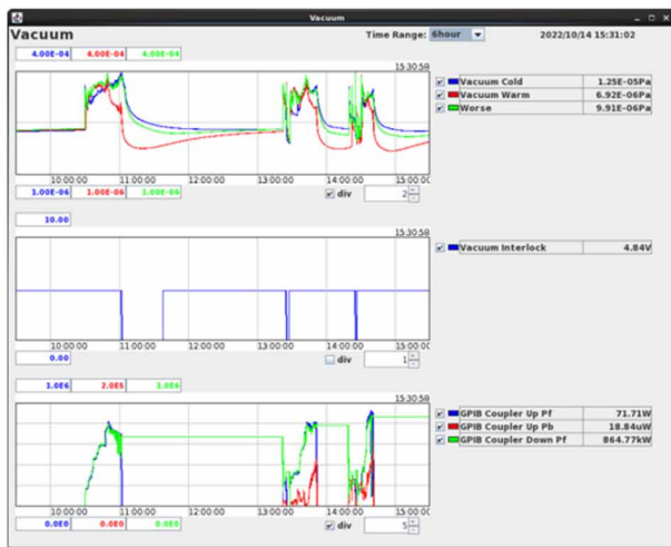
Figure 5: Trend of RF power, and the both vacuum during RF conditioning (left), and thermal cycle test (right).
