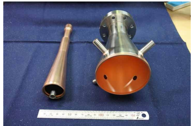
Figure 1: Mock-up of STF-type cold power coupler for the study of copper sulfate plating.
