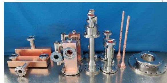
Figure 2: The fabricated 1.3 GHz (a) and 3.9 GHz (b) coupler prototypes.
