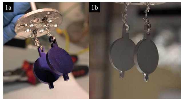
Figure 1: Nb 1'' circular targets mounted on the sample holder before (a) and after (b) dipping process. The blue colour (a) is due to the anodization process.
