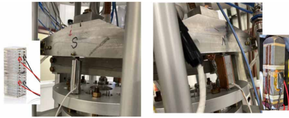
Figure 2: Close-up look at the location of the piezos on the cavity tuner.
