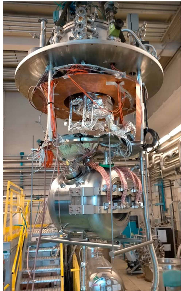
Figure 5: Cavity and its tuner equipped on the cold mass before insertion in the vertical cryostat.
