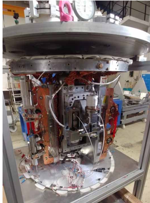
Figure 9: Motor cartridge installed on the cold mass before insertion in the liquid nitrogen cryostat.
