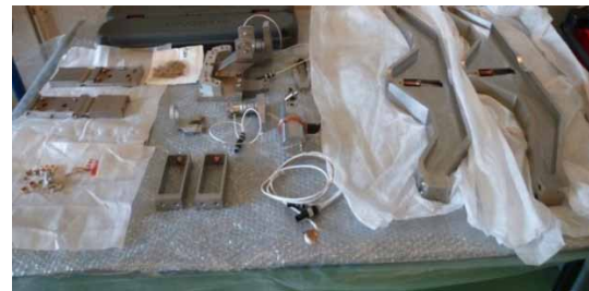
Figure 2: Every parts of the tuner before first assembling.
