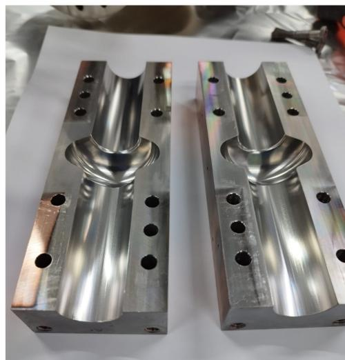
Figure 8: Photograph of the split 6 GHz cavity after deposition
