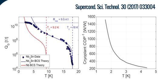
Bulk Nb has reached limit performance:  $Q_0 \sim 10^{10}$  @  $T_{op} = 2$  K with gradient closer to  $H_{sh}$
