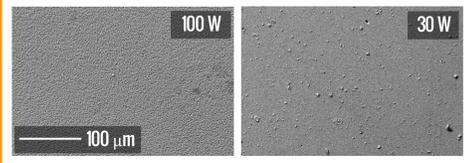
Increasing the process/annealing temperature mitigates tin clustering and affects  $T_c$  positively
