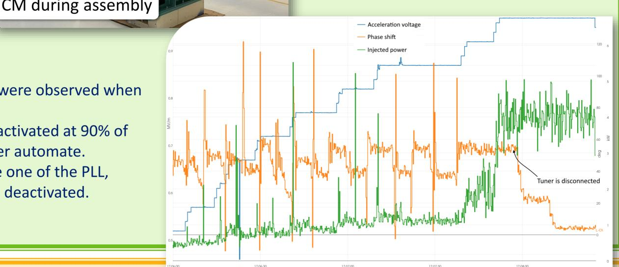
Despite some difficulties due to the vibrations of the tuner motors, all the requirements were successfully verified. Only one cavity required some conditioning to reach the target. The power consumption was compliant with the cryogenic requirements, even if the 6th cavity required a bit more than expected. The external quality factor of the couplers was compliant for all couplers.
