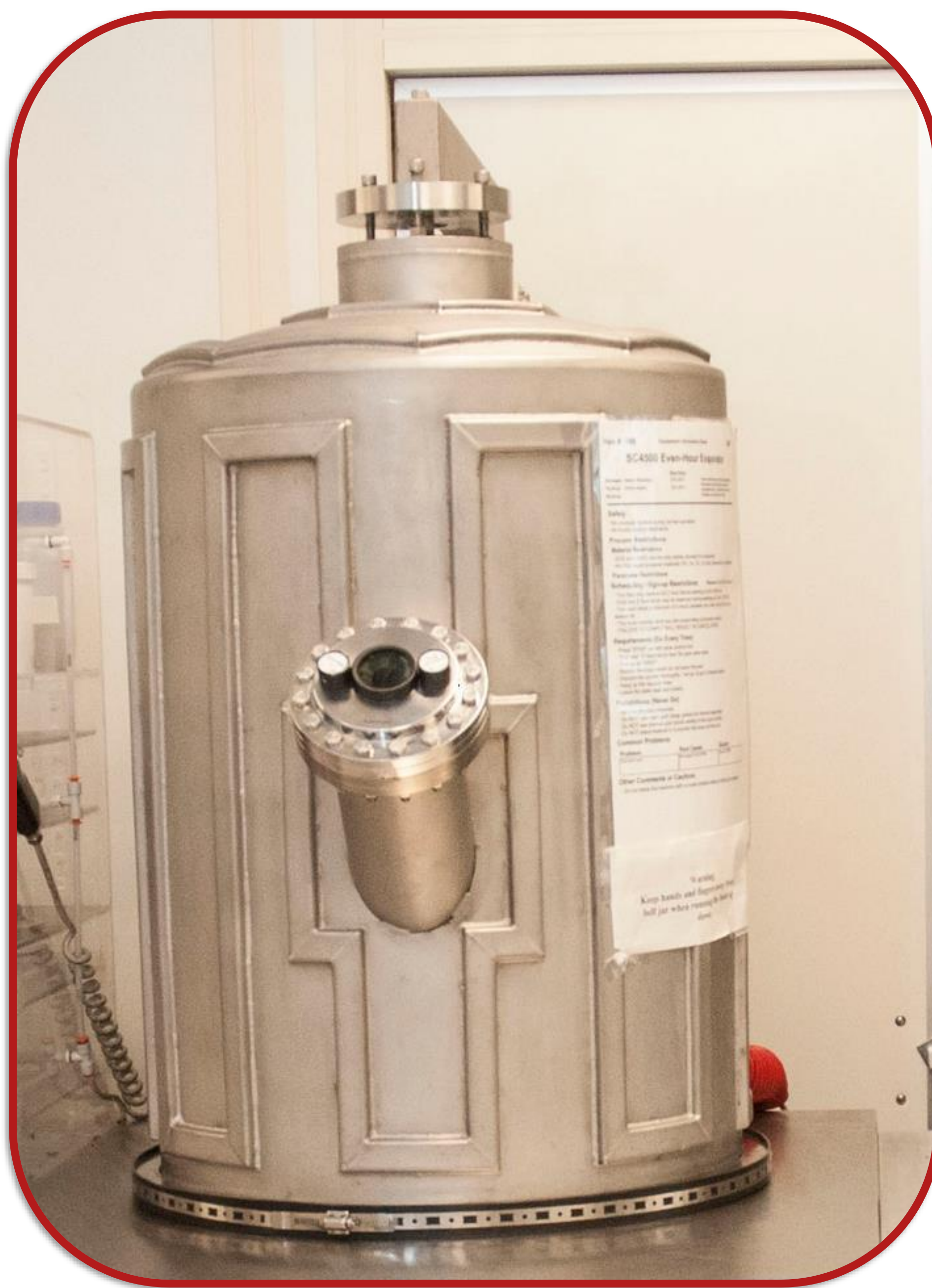
Above: CVC SC4500 evaporation deposition chamber, used to deposit thin gold layers.
