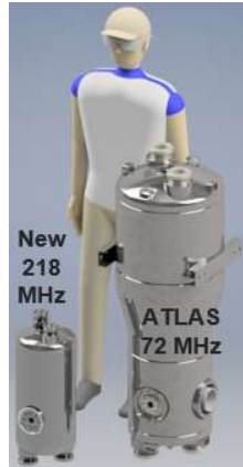
BCS surface resistance vs temperature plot (top left), accelerator cavity geometry regimes (bottom left), and example of physical scaling of cavity size vs frequency (right)
