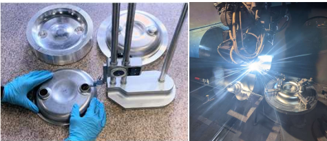
Cavity fabrication: niobium hydroformed parts (left, right), electron beam welding ports (middle)
