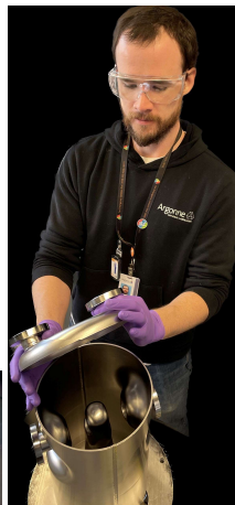
Cavity fabrication: niobium hydroformed parts (left, right), electron beam welding ports (middle)
