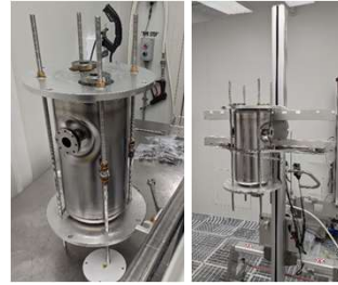
Photos of cavity ultrasonic and high pressure rinsing fixturing (left) and of the stainless steel helium vessel used for testing in Argonne's TC3
